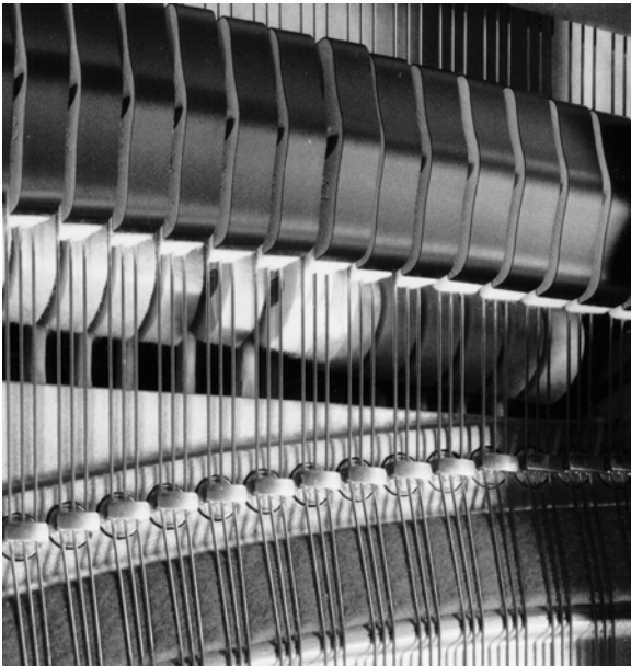
Figure 6: With felt under rollers, hammers may be blocked simply by pressing the key.
