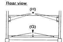
3. Hold (B) behind (A) and (C). Fasten (A) and (B) with four screws (H) and with three screws (G).
