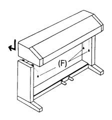
4. Place the piano on the stand. Then, slide the piano backward to place it at the appropriate point for screws. Hold the piano on the stand so that it doesn't fall from the stand. Then fasten the piano and the stand with four long screws.
