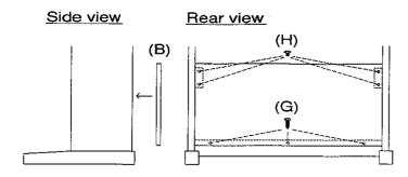
3. Hold (B) behind (A) and (C). Fasten (A) and (B) with four screws (H) and with three screws (G).
