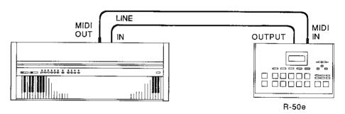
When connected as shown in the illustration, you can not only play along with the rhythm from the R-50e, you can also play the R-50e by striking the keys on the digital piano.
