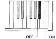
White key (ON): The piano will output sound when the keys are struck. Black key (OFF): Sound will be output only when MIDI data is received, and not when the keyboard is played.
