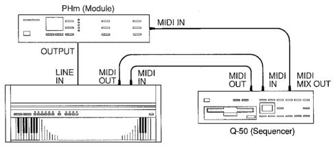
When connected as shown in the illustration, you can record songs played on the piano with the sequencer and play them back as many times as you like, and layer the module's tones made with the piano's MULTI TIMBRE function to assemble a complex automatic performance.
